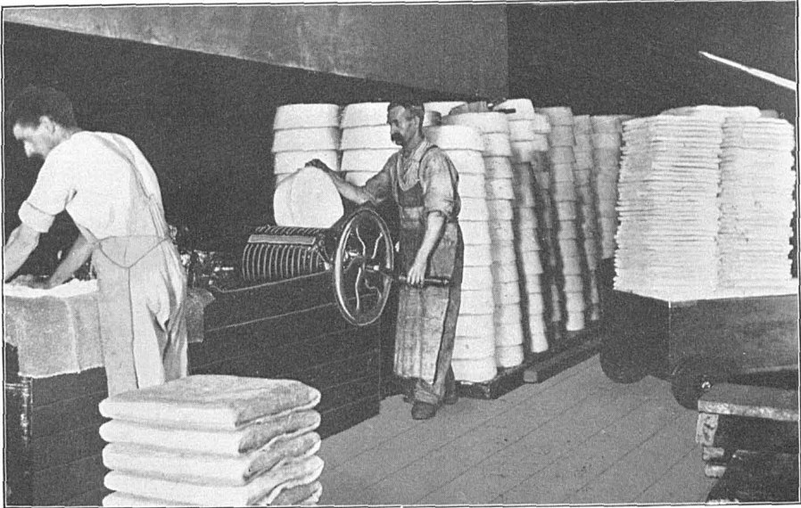
GRINDING AND PRESSING CRUDE SPERMACETI FOR REMOVAL OF TAUT-PRESSED OIL.
