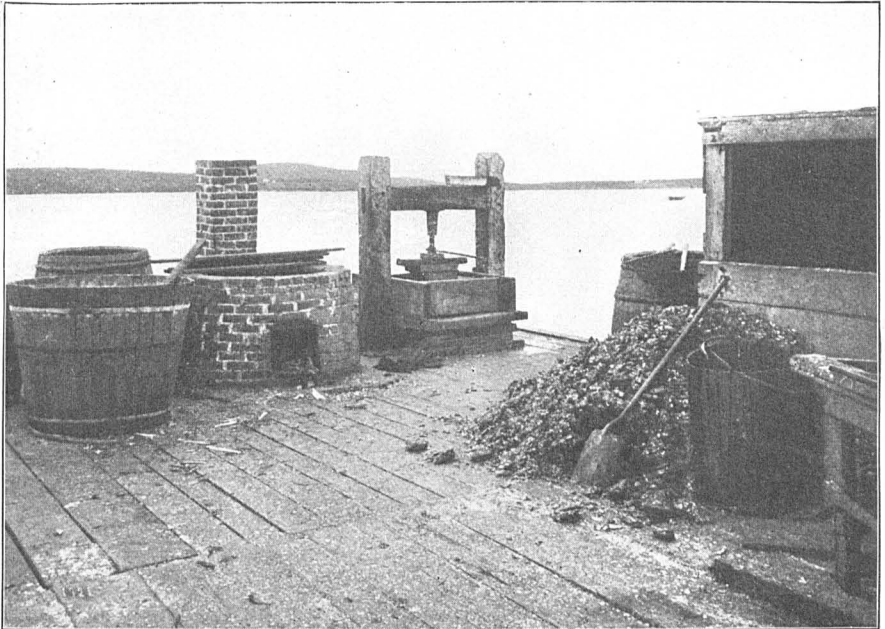
PRIMITIVE FORM OF KETTLE AND PRESS FOR RENDERING OIL FROM HERRING ON THE MAINE COAST.
