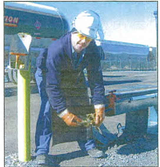
Albany, NY Propane Terminal Operator II John Houser demonstrates the quick and verifiable test for thread wear with the RMS ACME fittings test gauge, an innovation that raised the safety benchmark for the transfer of liquid propane.
